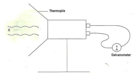
X is a radiation entering the thermopile. If the galvanometer needle shows a deflection,
