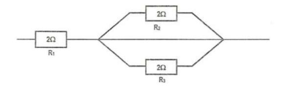
If the total current in the circuit is 2A, the potential difference across  $R_{\rm 3}$  is
