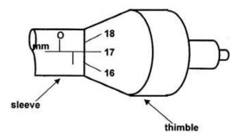
The reading on the micrometer gauge screw-gauge is • • •
